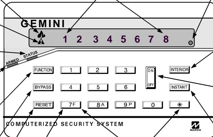
Press **INTERIOR** to bypass all interior protective devices such as motion sensors, etc.
