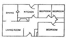
In homes with more than one sleeping area a smoke detector should be provided to protect each area. Smoke detectors shall be located between the sleeping area and the rest of the house. NOTE: Refer to N.F.P.A. 874 Appendix B1.1 through B-10.
